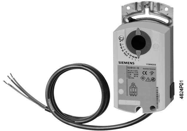
**Electric motor-driven actuators for three-position control, 5 / 10 Nm nominal torque, AC 24 V or AC 230 V operating voltage, mechanically adjustable working range between 0...90°, pre-wired with connecting cables of 0.9 m. Type-specific variations with adjustable auxiliary switches for supplementary functions or with potentiometer for position indication.**
