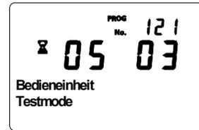
If the test was not successful, some other mounting location is to be selected or the AVS14.390 radio repeater can be used.
