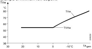
TVHw Minimum flow temperature setpoint TVw Flow temperature setpoint
