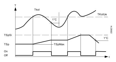
TSpSi Storage tank safety temperature TSp Storage tank temperature
