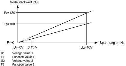
If the input signal drops below the limit value of 0.15 V, the heating demand is invalid and therefore has no effect.
