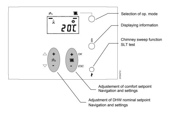
The above illustration shows an example of the front of an operator unit (not supplied as standard).
