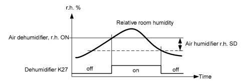
Relative room humidity is measured via any Hx input with the functions *Relative room humidity 10V.*
