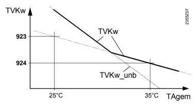
TVKw Flow temperature setpoint for cooling (with low limit control)
