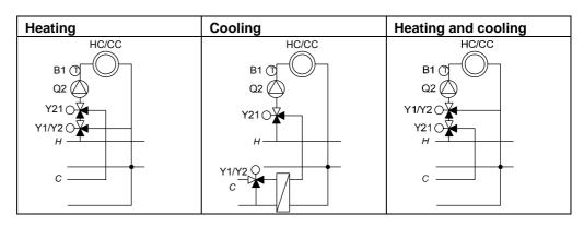
The setting is required when a QX... relay output (configuration) is used as a diverting cooling valve Y21.
