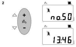
The display shows the first operating line, alternating with the value. Press the arrow button until you reach operating line "Hours / minutes" (e.g. 50).
