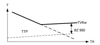
TVKw Flow temperature setpoint, cooling
