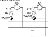
The cooling and heating circuits draw their cooling/heating energy from separate primary circuits.
