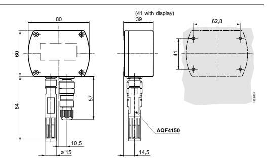
Dimensioning without (with) LCD-display
