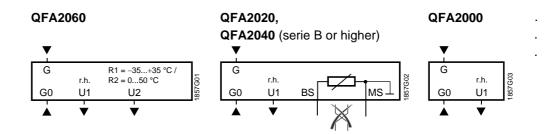
G, G0 Operating voltage AC 24 V (SELV) or DC 13.5...35 V U1 Signal output DC 0...10 V for relative humidity 0...100 %
