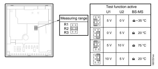
The setting element is accessible after removing the baseplate. It consists of 6 pins and a shorting plug. It is used to select the required measuring range and to activate the test function.
